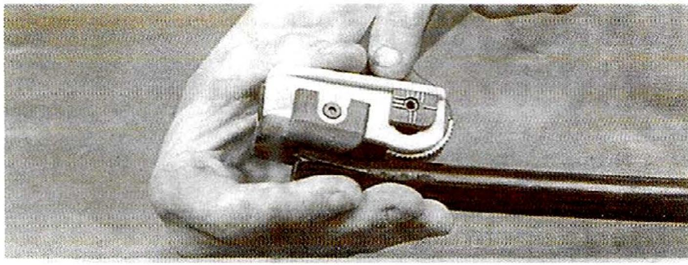
2 The eccentric unit has been adjusted correctly, if the plate of the cutter is parallel with the cable while the blade is inserted under the cable sheath.
