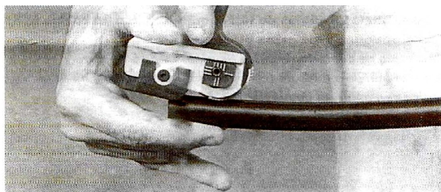
3 Set the blade of the cable sheath cutter so that it is located in the space between the conductor core units and the laminated cable sheath. Make the longitudinal cut by holding the cable against the serrated gripper and pressing down the hand lever.
